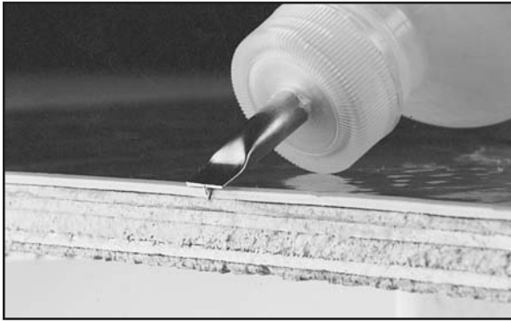
Fig. 7. Insert slotted fin into seam cut.
